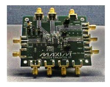
Objective: For the RF mixer in the FM (AMPS) signal path, to optimize the trade-off between best linearity versus highest gain by custom-tuning the output matching circuit.
